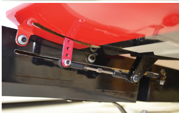
The elevator linkage has been installed. The adjustable pushrods make control surface adjustments easy.
