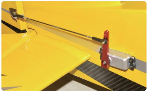
9.Insert the fiberglass control horn into the elevater, and glue with AB glue Screw the elevater servo onto the fuselage as shown.
