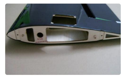
3.Use screw to lock the aluminum sheet onto the wings.
