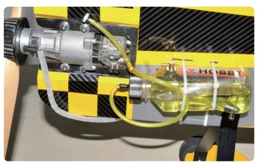
5.Screw the throttle servo onto the fuselage. Bent the pushrod, and use it to connect the servo and the engine.
