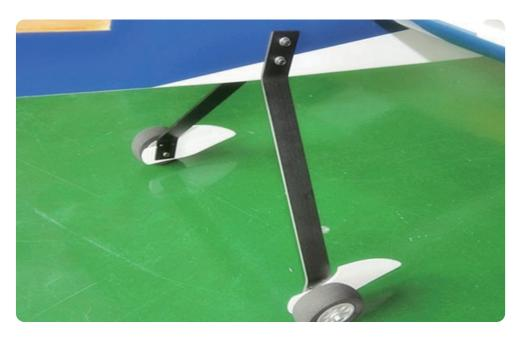
6.Drill a 6mm hole at the back tail of the fuselage to install the tail wheel
