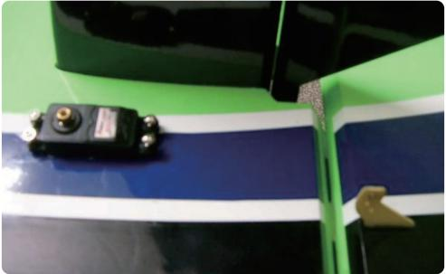
4.Connect the control horn and rudder servo with ball links and pushrod.
