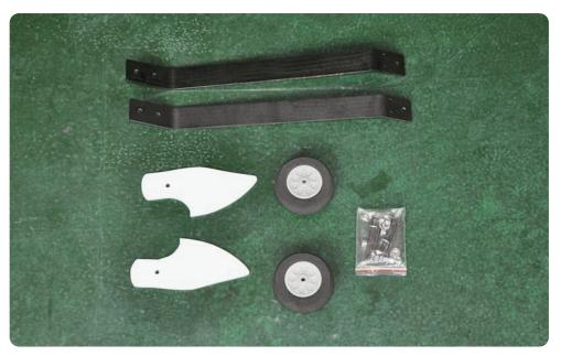
3.Use screw to connect the landing gear, wheel pant, nut and wheelin turn, and finally use a lock nut to lock them.
