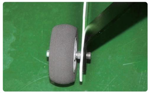
5.Use two screws to lock the two pieces of the landing gear to the fuselage
