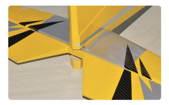
6.Insert the fiberglass control horn sheet into the aileron hole pre-cutted.Use AB glue to glue it.
