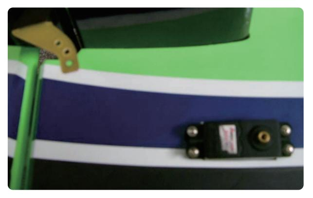
10.Connect the control horn and elevater servo with ball links and pushrod.
