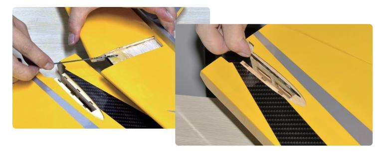
5.Use a saw to cut off the part at the end of the fuselage.
