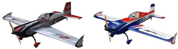
Wing Span:106in/2693mm; Flying Weight:11700g; Wing Area:138sq.dm; Radio:6Channel 11Servos; Length:94.5in/2400mm; Engine:100CC Gas
