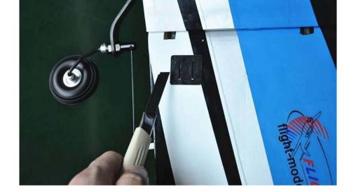
Insert the fiberglass control horn sheet and gear plates. Use AB glue to glue it.
