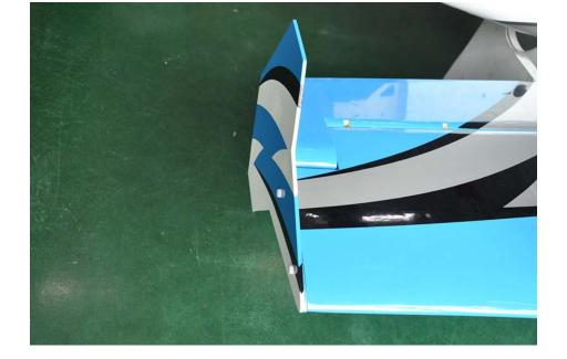
Connect the main wings and the fuselage with Carbon fiber tube.
