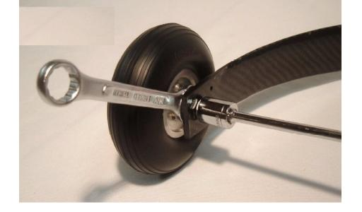
Install the wheel cover, and fix it up to landing gear with screw.
