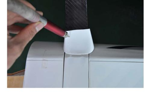
Use screws to lock the cuffer and landing gear
