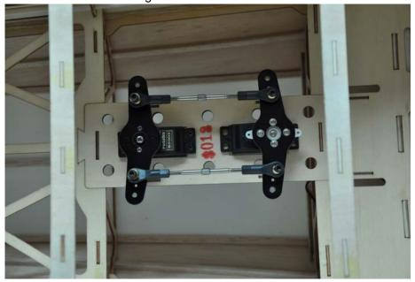
Use screws to fix up the servo on the fuselage
