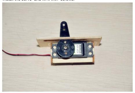
Use 3\*12 screws to lock the servo-tray to the Wing
