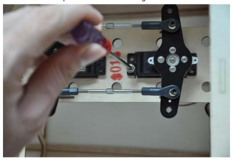
Attach the servo arm to the ruddert servo as shown
