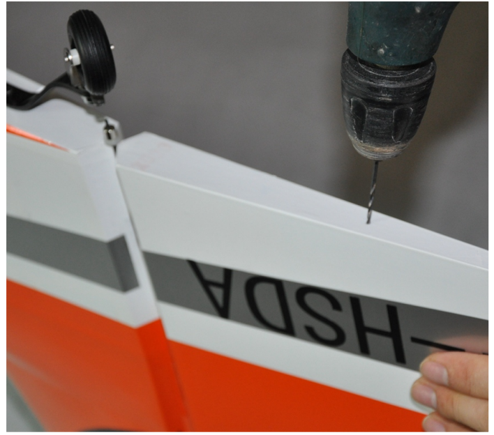
Drill the hole for install spring
