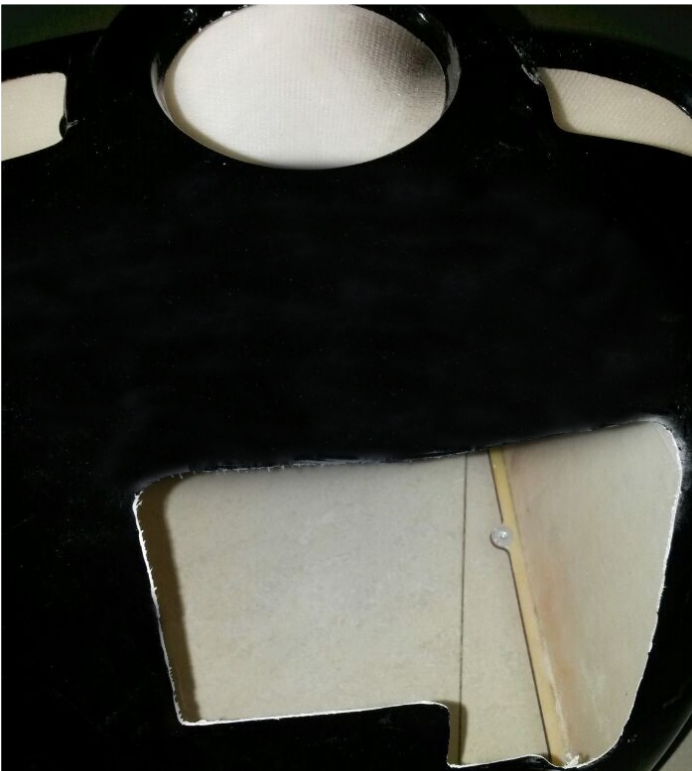
Cut a hole in the cowl for install Engine
