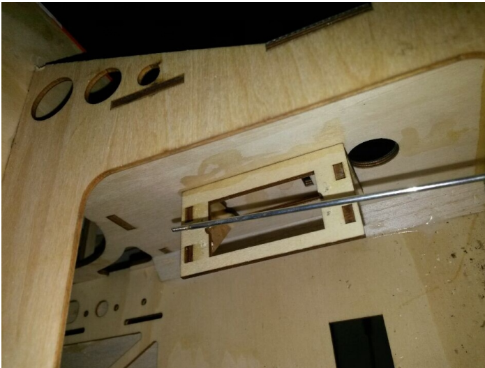
Install servo at the throttle
