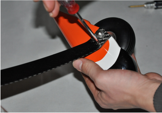
Install the wheel cover, and fix it up to landing gear with screw
