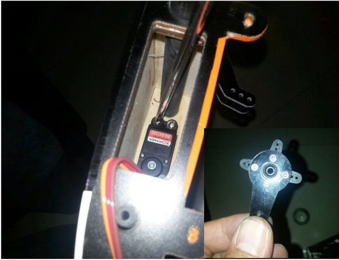
Install elevator servo
