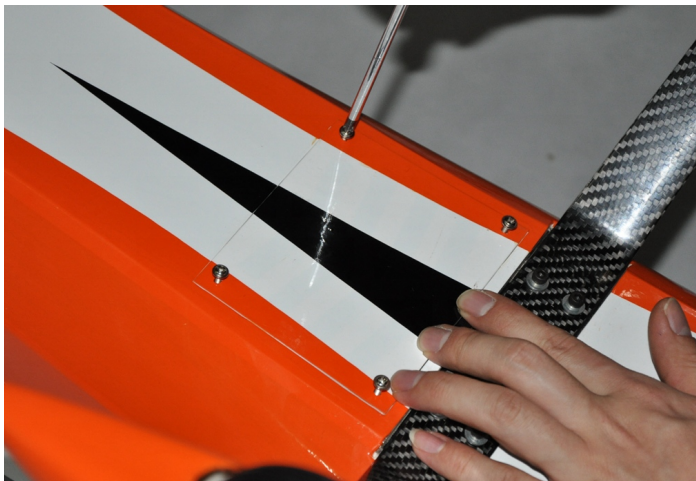
Install exhaust pipe plate
