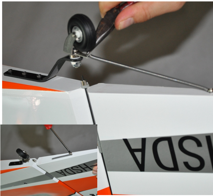
Connect the spring to the tail wheel
