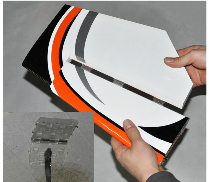
Apply epoxy into hinge hole of the wing
