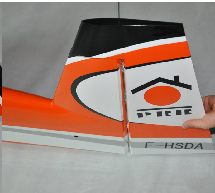
Put the steel wire in the hinges between the rudder and the connector of vertical fin
