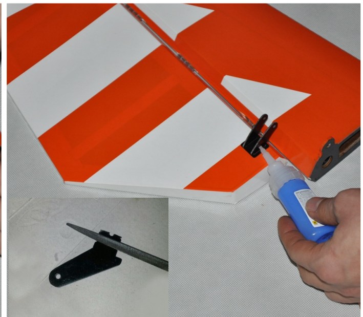
Insert the fiberglass control horn and glue with AB glue
