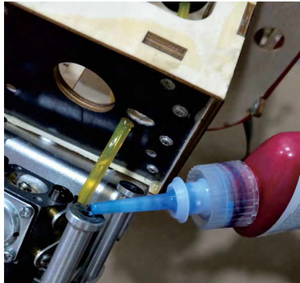
put the glue into the pillar of engine
