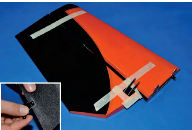
install the control-horn in the stabilizer
