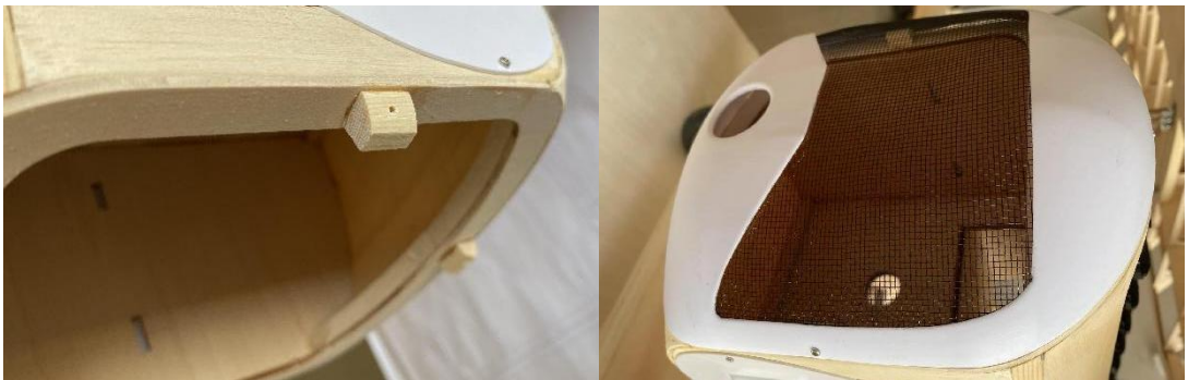
21) The pine block is attached to the nose to secure the cowling.
